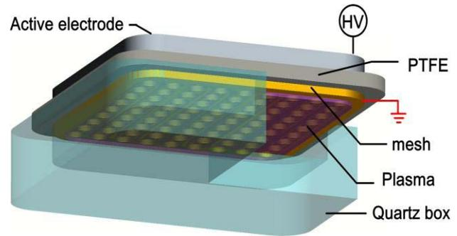
Fig. 1. Discharge device.
