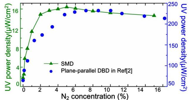
Fig. 2. Dependence of UV emission intensity on the N<sub>2</sub> concentration.
